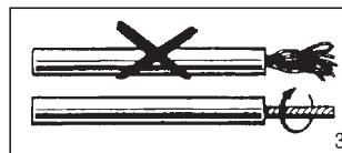
**Hint:** Twist the wire ends before inserting them into the terminal (Fig. 3).
