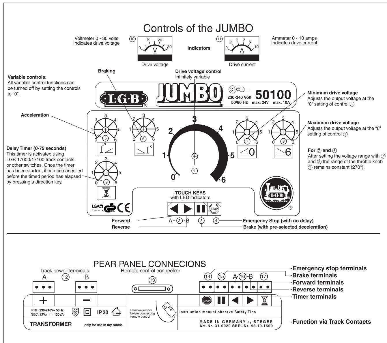
The JUMBO gives model railroaders enough power for large, complex layouts and multiple locos. You can use its features for automatic operation, for example, by using track contacts to trigger slow track sections or station stops.
