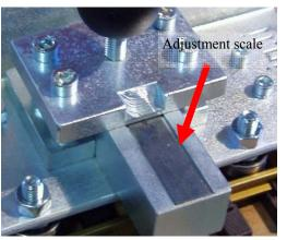
given millimetre reading and a radius of a curve. We could not provide this upfront, since the different rail materials (Brass, Stainless Steel, Nickel Silver, Aluminium) have different flex characteristics. This means if you bend a given piece of rail with the rail bender the metal will bounce back a little. How much depends on the material and the used ties.
